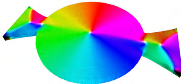
Figure 2.13: An example of the disk structure with contacts used in the micromagnetic simulations. The color gradient shows the IP rotation of the magnetic moments, forming a vortex state.
