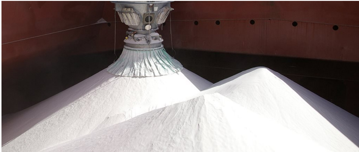
Figure 2: Alumina - Aluminumoxid: Raw Material for the production of primary aluminum (Norsk Hydro, 2020a).
