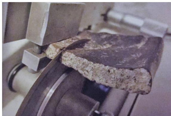
Figure 26: Cutting off a chip from a ceramic sherd in order to make a thin section (Quinn 2013, 24).
