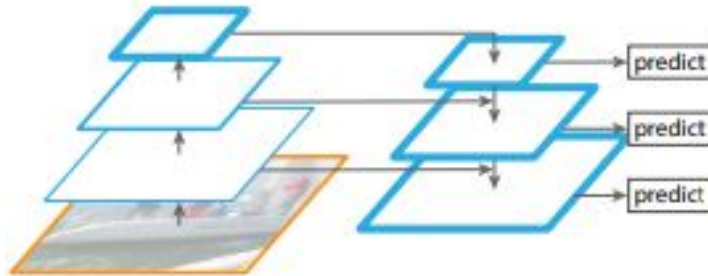
Figure B.11: Feature Pyramid Network) (Lin et al. 2017); the arrows represent the bottom-up, top-down and lateral connections
