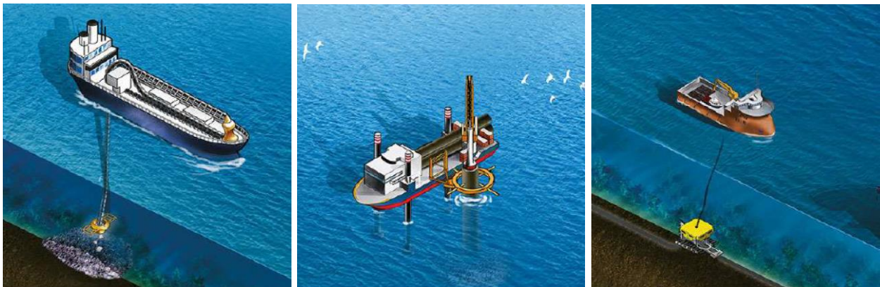
figure 4.15 - Illustration of seabed preparation (left), monopile piling (middle), and cable laying (right) (geminiwindpark.nl).
