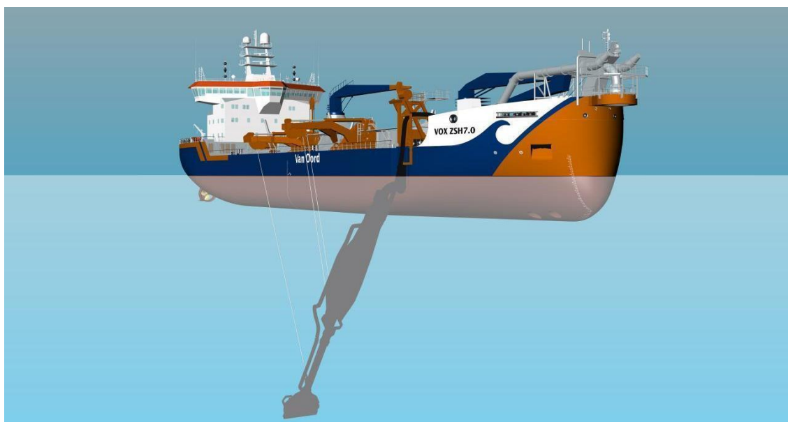
Figure 4.8 - Illustration of one of Van Oord's newest trailing suction hopper dredgers (vanoord.nl).
