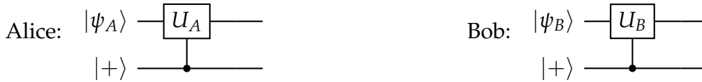
Figure 2.6: Alice's (left) and Bob's (right) circuits when the controlled gates used are Haar unitaries.
