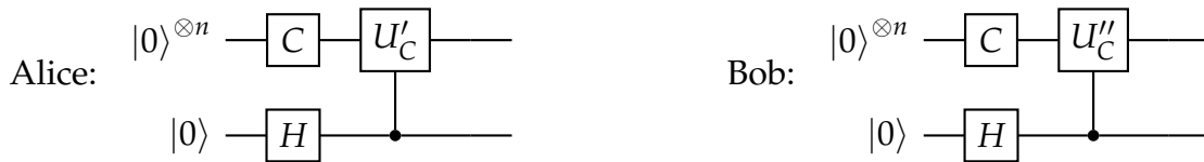
Figure 2.3: Alice's (left) and Bob's (right) circuits for the implementation of a cross-platform verification algorithm using Z gates on the controlled-unitaries, U'_C , U''_C , being the Z gate applied on a different qubit on each unitary.
