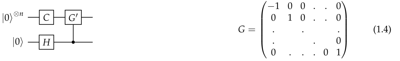
Figure 1.2: Cross-platform verification protocol based on Grover search reflections, where G' = C^\dagger G C , is a reflection with axis C|0\rangle .
