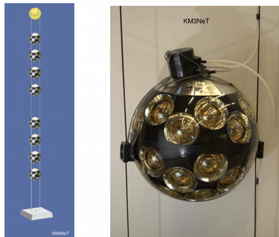
Figure 3.2: On the left, a representation of one string. On the right, a singular DOM consisting of 31 PMTs [20].
