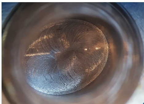
(a) Trap as seen from above through a microscope, just after cleaning it. Showing the elliptical shape and the clean bottom.
