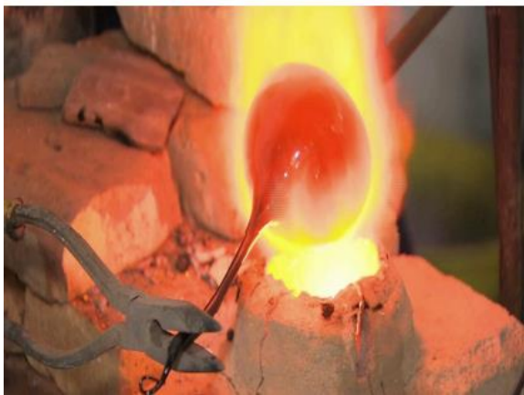
Figure 1.1: Drawn glass created by using the Lada-method (picture by Lankton, after figure 18 in Pion 2014a, 38).
