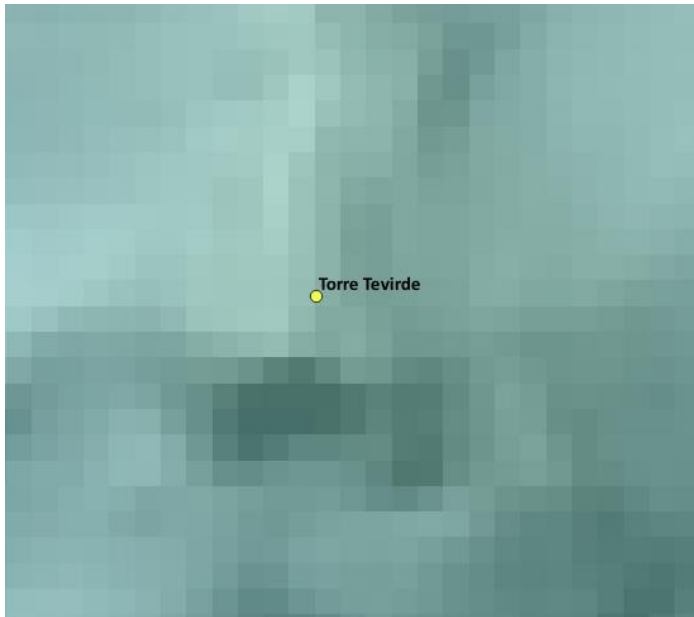
Figure 25. An example of the cells when zoomed in. Every cell is 5 by 5 meters (by author).
