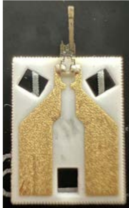
Figure 3.6: Probe with broken tuning fork for short test. There are only two silver epoxy contacts on the tuning fork, which are covered with Torr seal. Then the probe was covered with the Kapton mask for sputtering, which turned out to be insulating.
