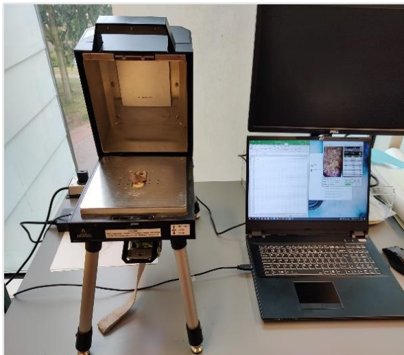
Figure 8: PXRF equipment. The PXRF scanner is inserted in a small chamber to isolate the radiation (Photo credits: author).
