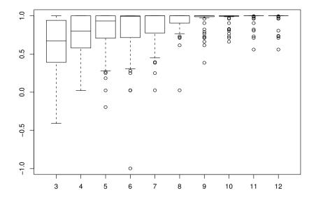
Figure 2: Results of performing 50 experiments on a very small design consisting of 4 switches, where the test runs were chosen randomly, but without repeating a single switch setting for more than one test run. The x axis gives the number of test runs, and the y axis gives an indication of the true quality of the switch setting which was expected to be optimal at that point. The true optimal setting is at 1, and the general mean is at 0.
