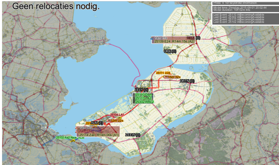
Figure 15: The interface of TIFAR. The base locations are indicated with with names, and the number between the brackets are the number of ambulances at the base. Ambulances responding to an incident follow a red route. In the top left is shown which relocation should be taken, if any.
