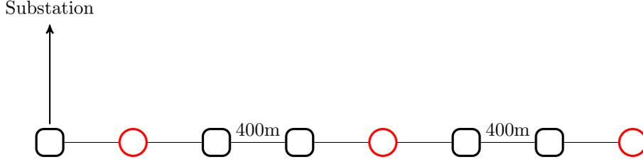
Figure 12: Representation of an outer branch of the distribution grid with the characteristic length between joints. The red circles are connections to lower parts of the grid or customers. The black rectangles represent the cable joints. The cable joints are modeled as part of the edges.
