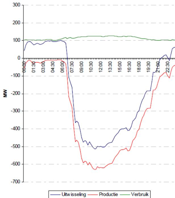
Figure 4: The load profile of the distribution grid of Westland Infra at 2 June 2011. The green line is the consumption and the red line the production. Both lines represent power flowing from the transmission grid into the distribution grid, hence the production is negative. The blue line is the exchange between the transmission grid and the distribution grid, which can be acquired from adding the production and consumption. The figure is obtained from [7].
