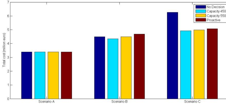
Figure 27: Total cost in million euros for the four different maintenance models under the different scenarios.
