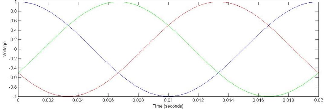
Figure 1: Voltage profile of a three phase power flow with  $V_{\max} = 1$  and a frequency of 50 Hz. The blue line has no phase shift, the green line is shifted 120 degrees and the red line has a 240 degrees phase shift.
