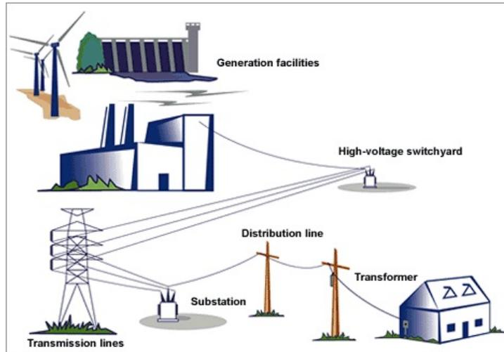
Figure 2: Schematic view of the distribution of electricity.
