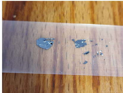
Figure 3.7: \text{MoS}_2 crystal on scotch tape. This tape could serve as a mother tape for the exfoliation process of \text{MoS}_2 .
