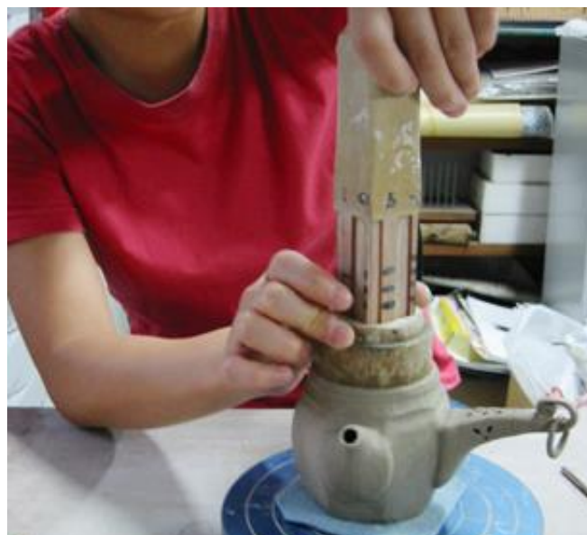
Image 8. A mould being removed
