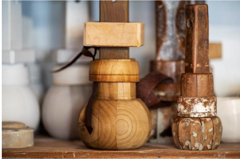
Image 5. Constructed kigata Banko moulds
