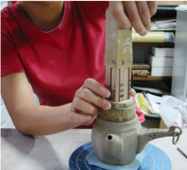
Image 8. A mould being removed
