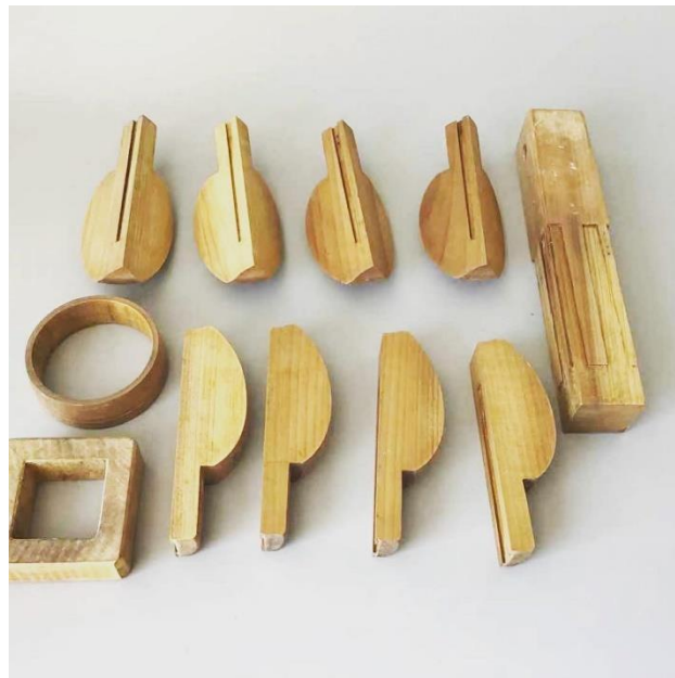
Image 6. Deconstructed Kigata Banko mould.
