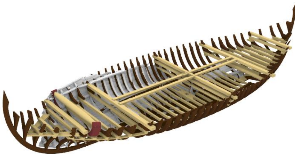
Figure 75 The model of the Big Ship of Wismar including the transverse beams and windlass. Brown indicates oak. Sand colour indicated pine. Red indicates elm. (Hernandez Montfort based on the model by Ditta & Auer, in press).
