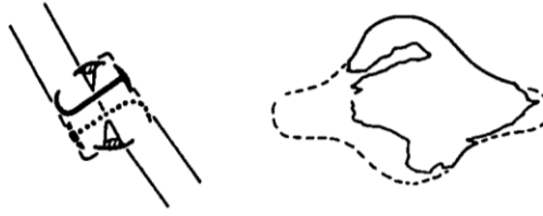
Figure 6 The butterfly-shaped iron staple ( sintel in Dutch) used in later cogs. (Reinders, 1985, fig. 8).
