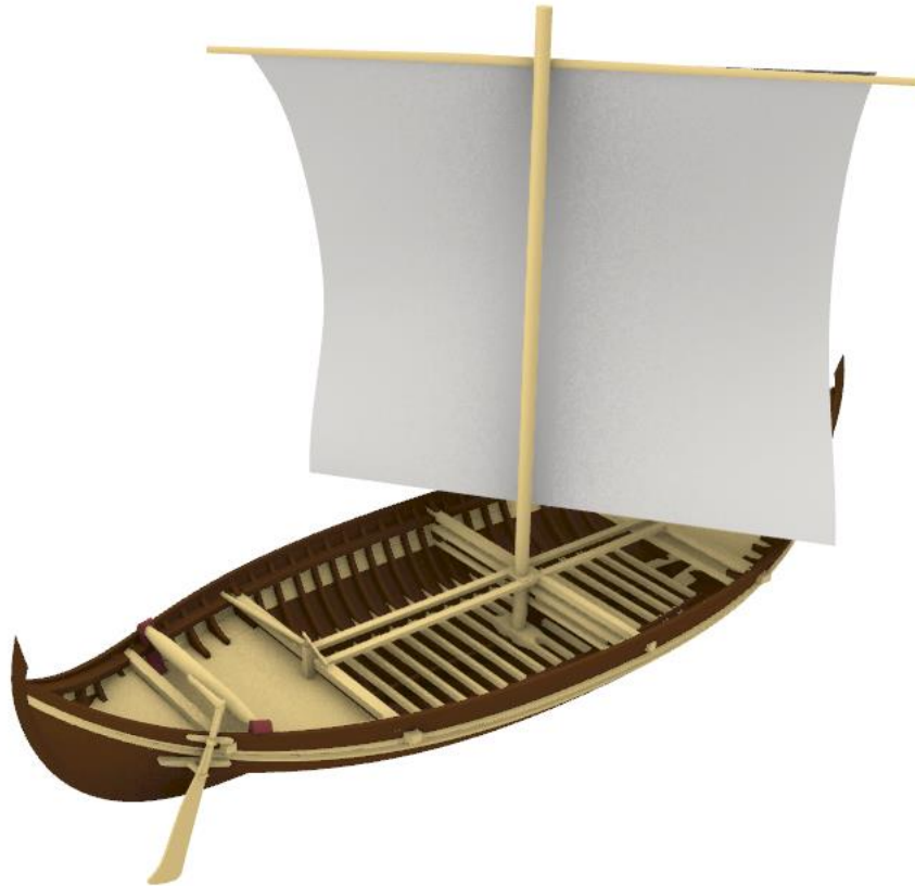
Figure 84 The model of the Big Ship of Wismar with mast, sail, rudder, and pump. Brown indicates oak. Sand colour indicated pine. Red indicates elm. (Hernandez Montfort based on the model by Ditta & Auer, in press).
