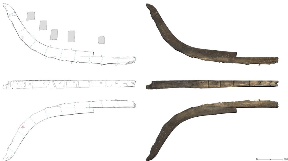
Figure 70 Biti and biti knee connection. The oak biti knees rest on top of the pine bitis and are attached with treenails. (Taken from Auer & Ditta, 2019, timbers 203 (biti) and 303 (biti knee)).
