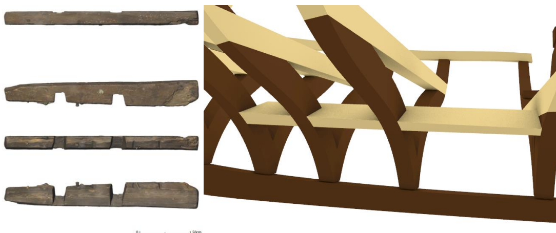
Figure 72 The lower pine stringer aft of the keelson. These pine stringers are cut out to fit the floor timbers and provide longitudinal strength as an extension of the keelson. Left: photography of a preserved lower stringer. Taken from Auer & Ditta, 2019, timber 221. Right: Reconstructed 3D model showing the position of the lower stringer. Brown indicates oak. Sand colour indicated pine. (Hernandez Montfort based on the model by Ditta & Auer, in press).
