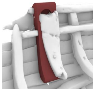
Figure 76 Model of the windlass knee. The model of the windlass knee (red) against the scanned model of preserved timbers (white). (Hernandez Montfort, model by Ditta & Auer, in press).
