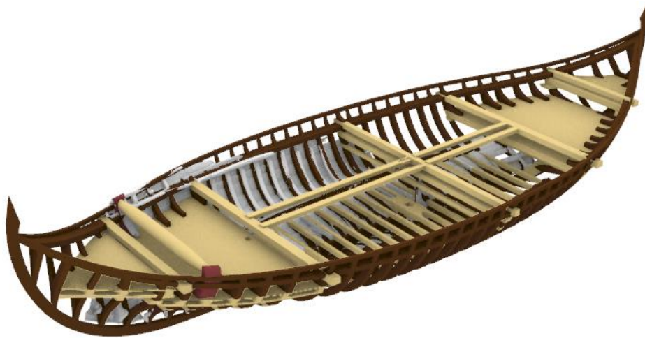
Figure 80 The model of the Big Ship of Wismar with the upper stringers. Brown indicates oak. Sand colour indicated pine. Red indicates elm. (Hernandez Montfort based on the model by Ditta & Auer, in press).
