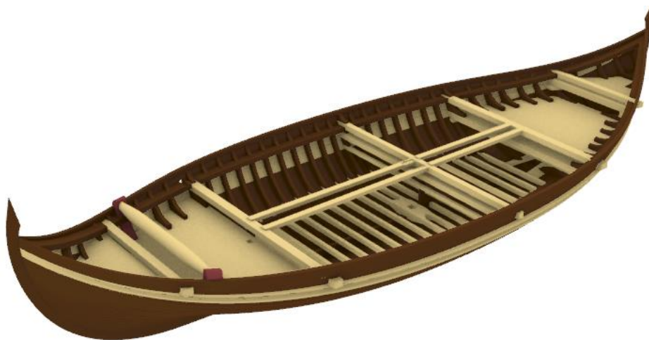
Figure 81 Model of the hull including outer planking. Brown indicates oak. Sand colour indicated pine. Red indicates elm. (Hernandez Montfort based on the model by Ditta & Auer, in press).
