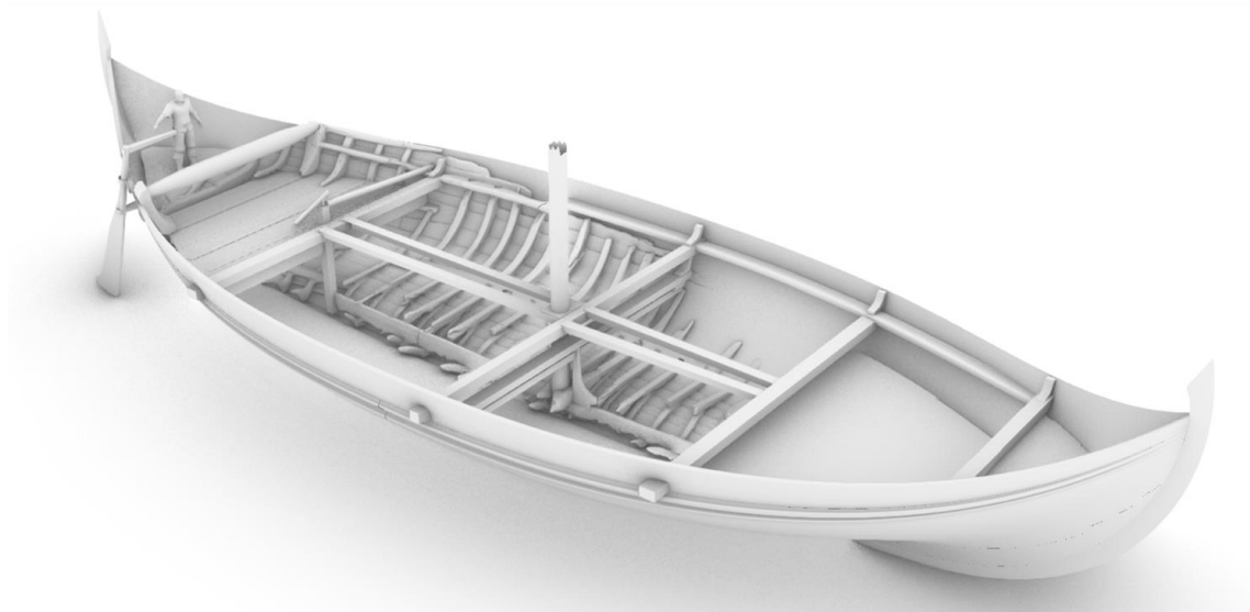
Figure 43 Visual reconstruction of the Big Ship of Wismar. Both the scanned model of the preserved timbers and the visualization model are shown here. (Figure by Hernandez Montfort, model by Ditta & Auer, in press).
