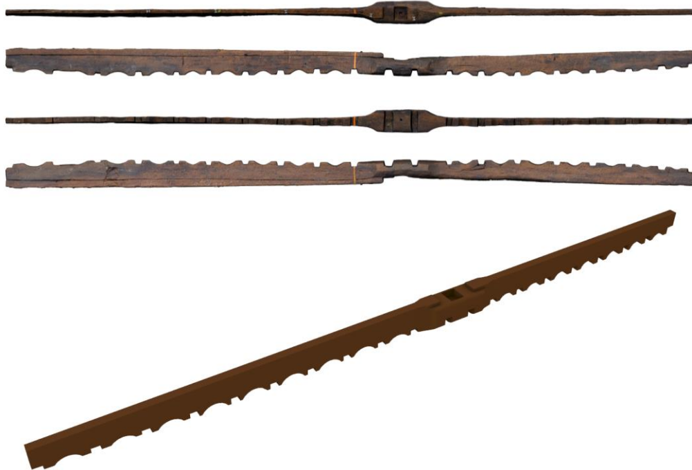
Figure 65 The Keelson. Top: photograph of the preserved keelson. (Taken from Auer & Ditta, 2019, timber number 211). Bottom: 3D model of the reconstructed keelson (Hernandez Montfort).
