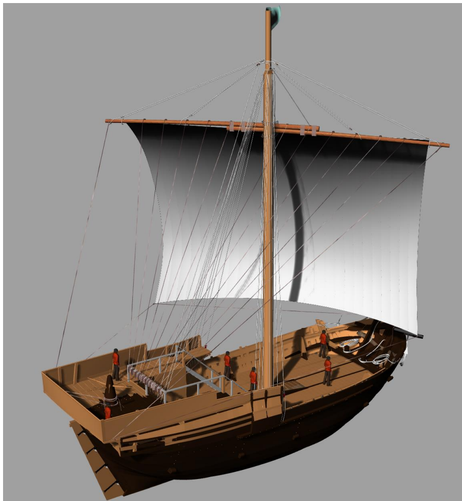
Figure 53 The highly detailed 3D model of the Bremen cog. Dark timbers represent preserved timbers. Light brown timbers are reconstructed. (Figure by Hernandez Montfort after model by Tanner, 2018).
