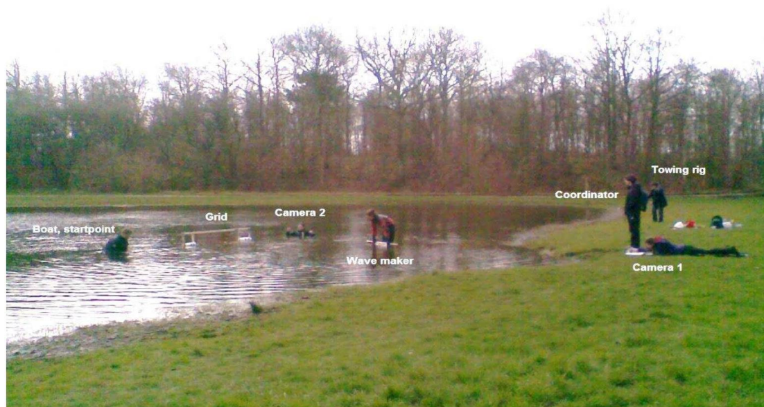
Figure 30 Model tests set-up in a lake. (Ejstrud, et al., 2012, pp. 36, fig.17).
