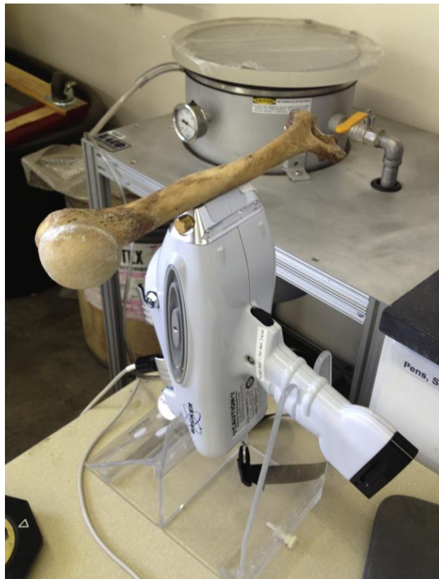
Figure 7: pXRF set-up by Perrone et al. The bone is balanced on top of the sensor. (Perrone et al., 2014, p. 151).
