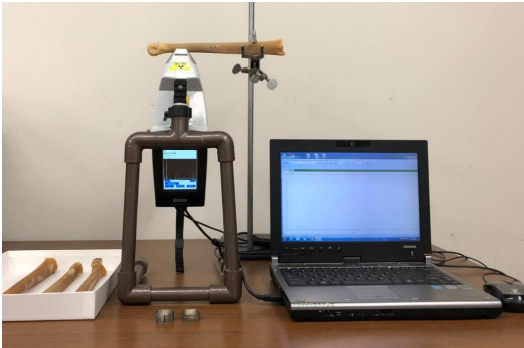
Figure 8: pXRF set-up by Henderson 2019. The bone is balanced on top of the sensor, but with additional support. (Henderson, 2019, p. 30).
