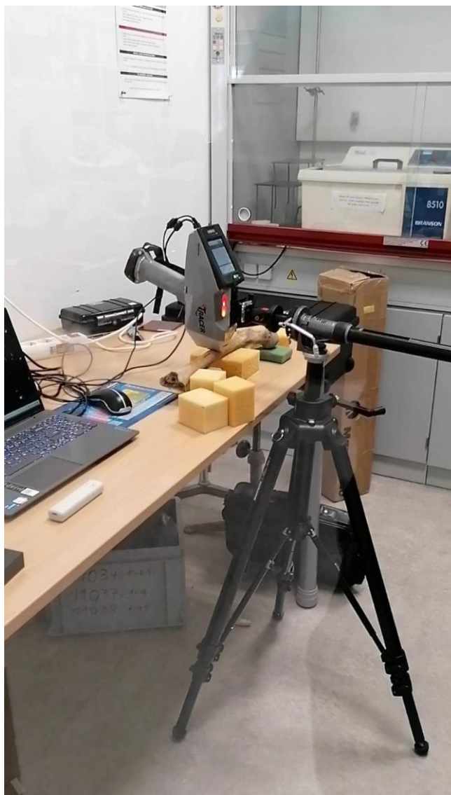
Figure 13: pXRF set-up in the current study. The bone is scanned in a top-down fashion by a pXRF supported on a tripod. (Photograph by Martijn Jacobs).
