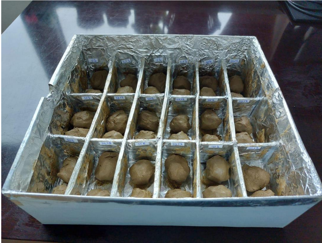
Picture 3: Picture of the organiser box lined with tin foil, containing all samples in their accordingly labelled compartments. This picture was taken just prior to a round of experiments, so the samples have been taken out of their individual storage bags already and kneaded with a bit of water to make them easily kneadable again.
