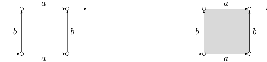
Figure 1: To the left an automata where its language represents the interleavings of the strings "a" and "b" and to the right a HDA where its language represents the parallel composition.
