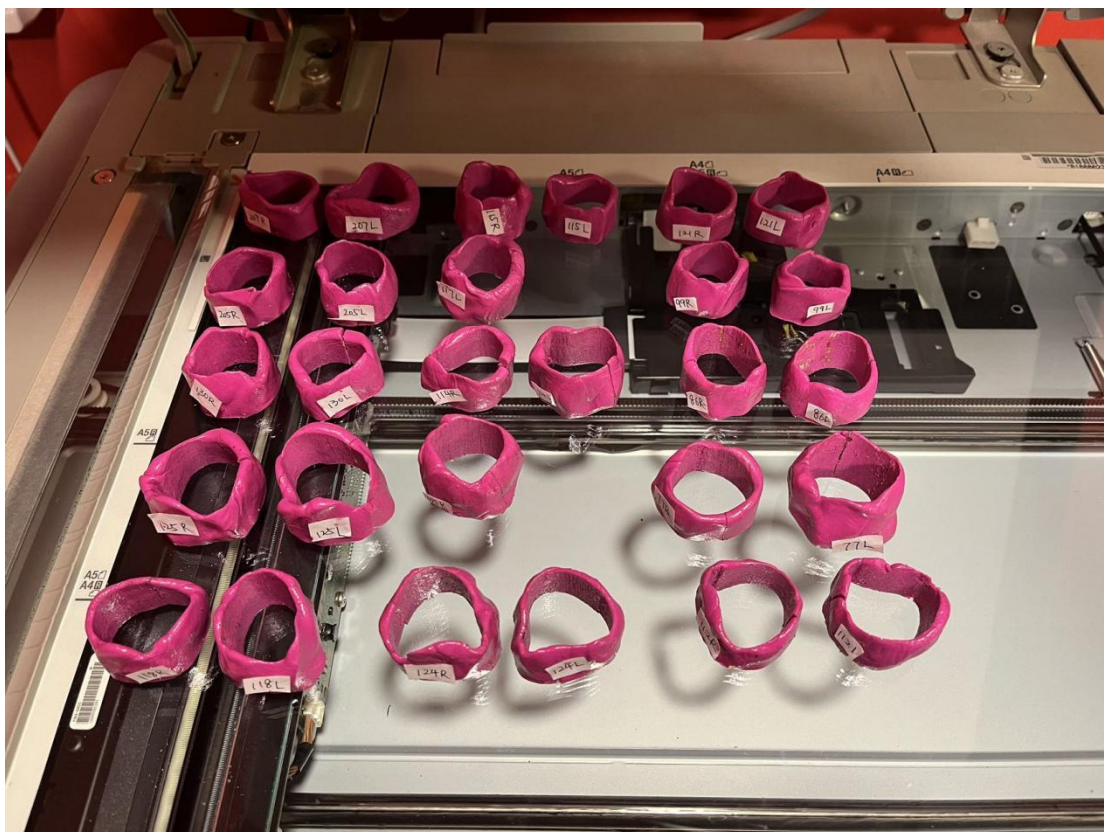
Figure3.2 Scan the outer contour lines of the cross-section (Photo by Xuwen Yue, 2023)
