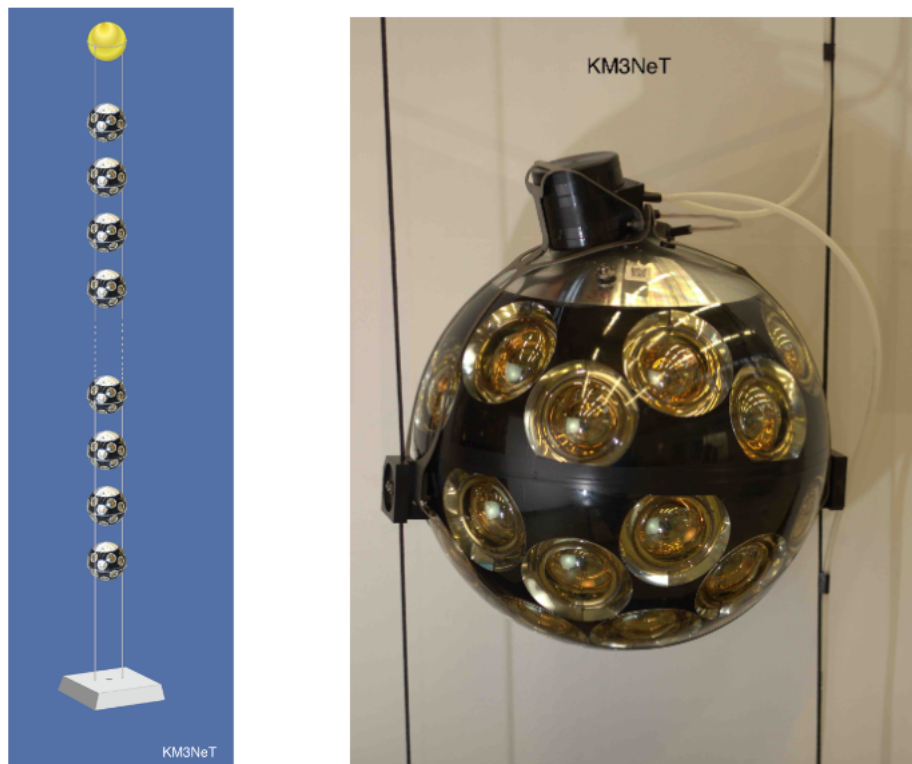
Figure 2.1: Left: image of a DU. In reality there are more DOMs located in a string. Right: a single DOM. Visible are the various PMTs, the electrical-optical cable on top, and the two titanium collars on the sides holding the rope supporting the DOM. Picture obtained from [6].
