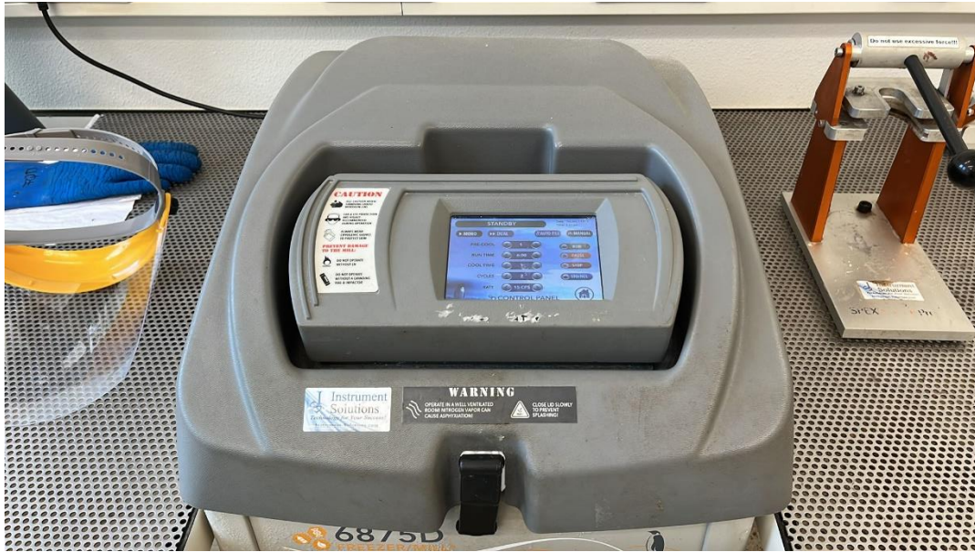
Figure 3.15: Photograph of the 6875D Freezer/Mill® Dual-Chamber Cryogenic Grinder. On the left side of the picture the cold-proof safety gloves and safety mask can be seen. On the right side, the device used to open the cannisters can be seen. Photograph by Author, 2022).
