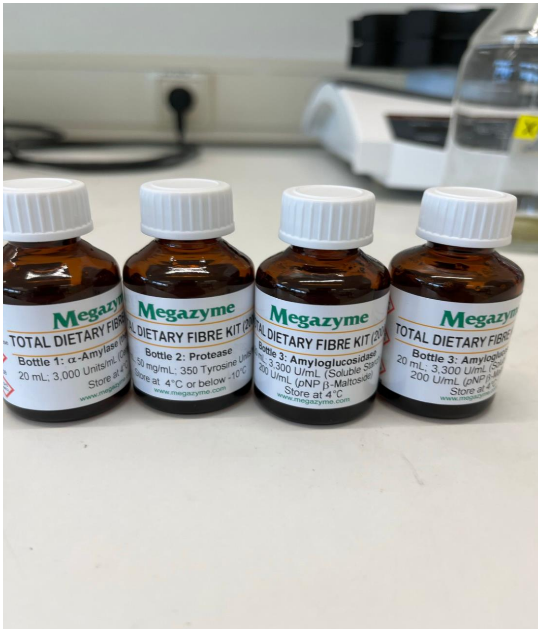
Figure 3.21: Photograph of all enzymes used for the TDF analysis, according to the TDF Assay Procedure K-TDFR-100A/K-TDFR-200A 04/17 manual. Photograph by Author, 2022.
