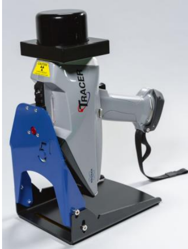
Figure 9. The pXRF instrument on its desktop stand, facing upwards, with the lid on (Bruker, n.d.).
