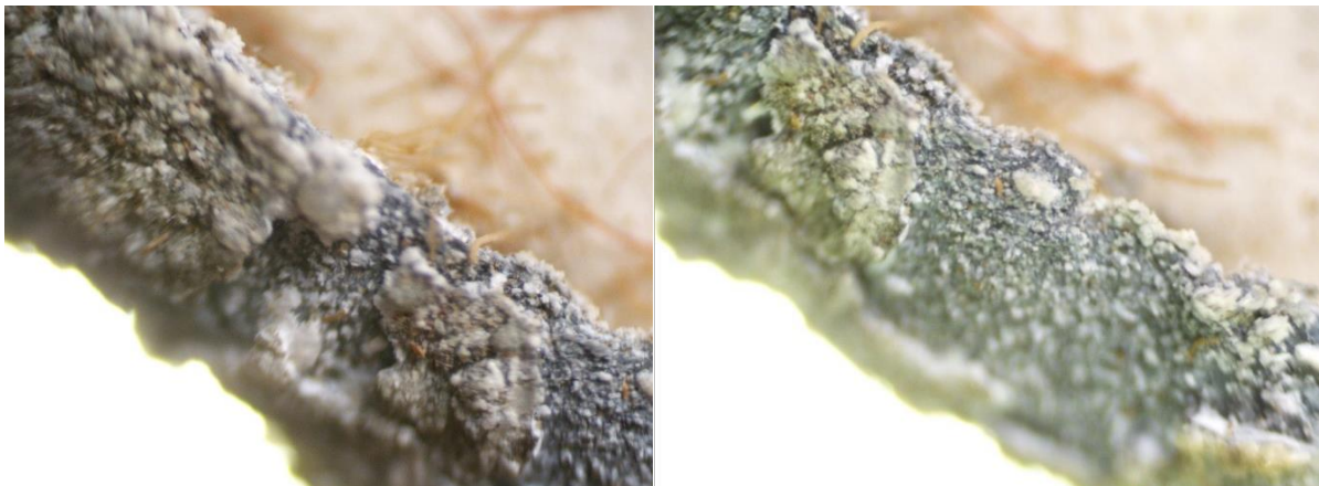
Figure 16. A microscopic view of the pin shows the corrosion and tiny sand particles on the metal frame.
