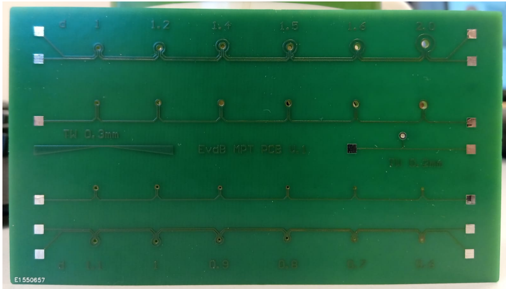
Figure 3.2: A photograph of the front side of the Printed Circuit Board with our design for many differently sized double-loop configurations and (anti)Helmholtz configurations, which makes use of printing the second loop on the other side of the board. The loops with a larger diameter are printed with a track width of 300\mu\text{m} , while the smaller traps are printed with a track width 200\mu\text{m} . The track height is 30\mu\text{m} copper. Board material is standard FR-4. Our measurements were done in the 1.4\text{mm} wide double-loop trap.
