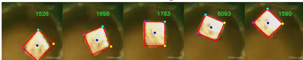
(c) Five consecutive frames taken during motion tracking of the levitated cube magnet's motion. The object detection method is used here. We see that for every frame the tracker finds a rectangle shaped contour around the top of the cube, which is clearly visible in every frame. By tracking the location of the corners of this rectangle, we find its rotation around the z-axis, \alpha . This rotation has a low frequency, however, and can be well approximated by eye. The blue dot is the center of mass of the rectangle, whose coordinates are used in analyzing the x- and y motion. The number printed in green is the number of frames the software can analyze per second and is, due to the low computing power necessary for this method, simply bottlenecked by the speed of the video.
