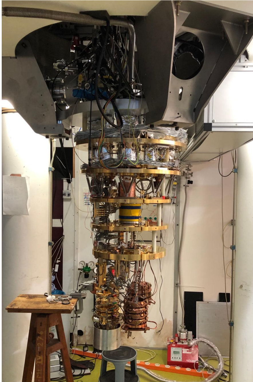
Figure B.2: Photograph of the CF1400 cryostat from Leiden Cryogenics in the Bouwmeester/Oosterkamp lab. The horizontal plates from top to bottom are at increasingly low temperatures starting from 50 K to 10 mK at the bottom of the cryostat. The cavity with the membrane-in-the-middle setup is attached to one of the Eddy current vibration isolators at the bottom. The mK temperatures are achieved using ^3\text{He}/^4\text{He} dilution.
