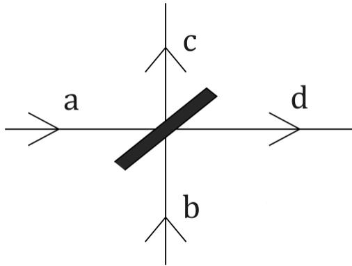
Figure 2: A schematic drawing of a beam splitter.
