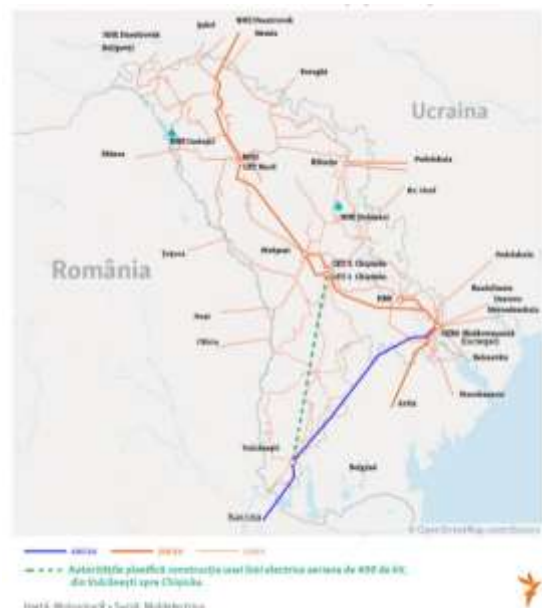
Figure 5: Direct high-voltage powerline between Vulcanesti and Chisinau (bypassing Transnistria and MGRES). Source: Radio Europa Liberă Moldova.
