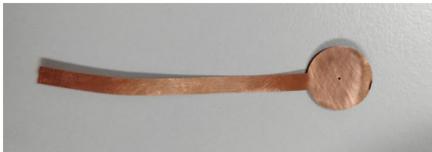
Figure 3.3: Thermalization foil for the microsphere
