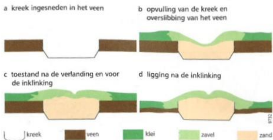
Figure 2.5, Schematic development of the formation of creek ridges. a= active tidal channel, incised in the underlying peat, b= backfill of the active tidal channel and the over silting of the peat, c= situation after the land dried up and before subsidence, d=placement after subsidence (Stouthamer, 2023, p. 295, Figure 11.7).
