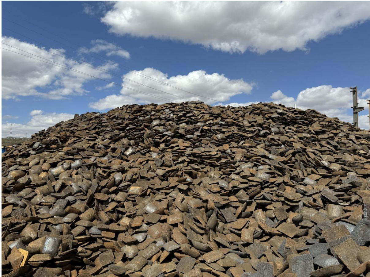
Figure 1.2: Photo of Blast Furnace Pig Iron. Dinson Iron and Steel Company Zimbabwe
