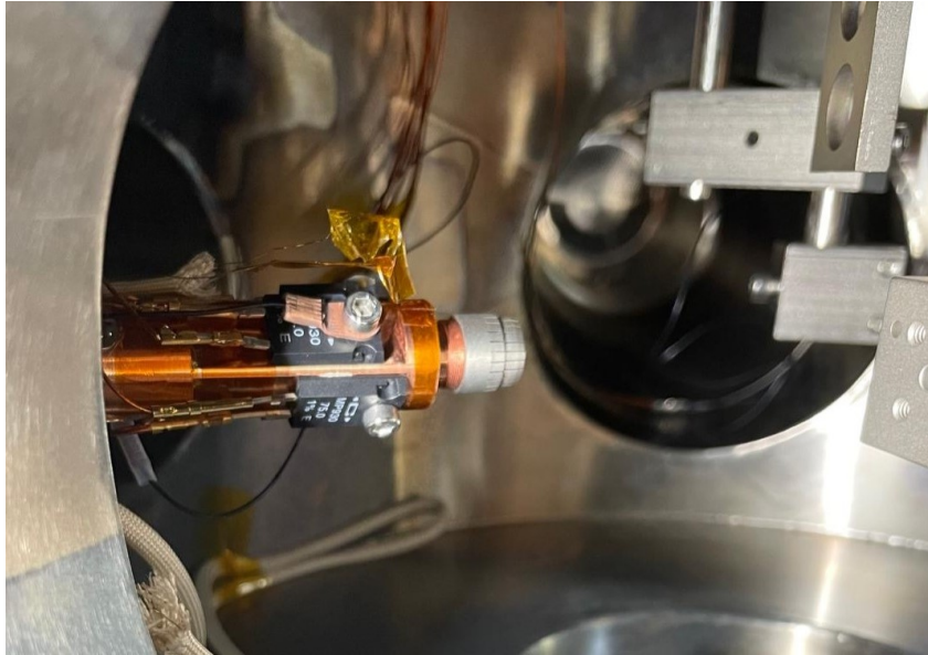
Figure 3.11: The transfer arm extension installed inside the prep chamber.
