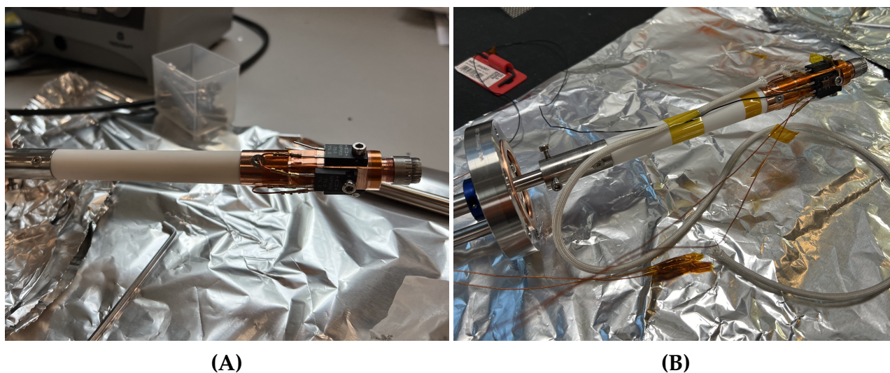
Figure 3.10: The custom transfer arm extension made in collaboration with the FMD and ELD. (A) Before wiring, but with the heating resistors screwed on. (B) Transfer arm after wiring of heating element, ground and TC.
