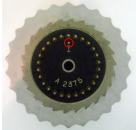
Figure 17: Enigma dot on rotor
