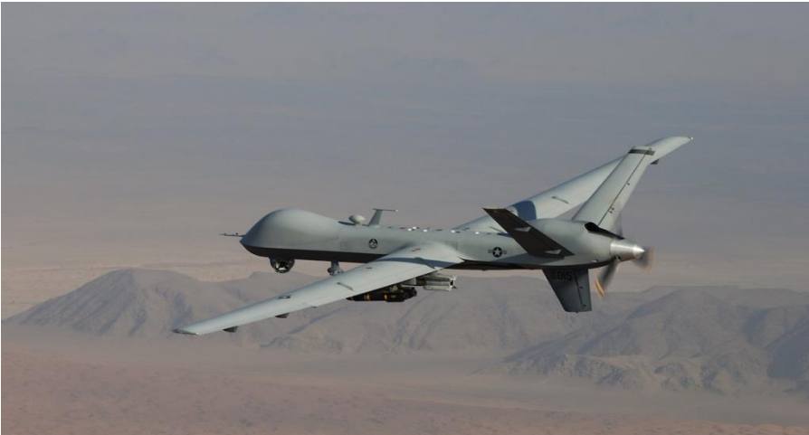
An MQ-9 Reaper , armed with GBU-12 Paveway II laser guided munitions and AGM-114 Hellfire missiles, piloted by Col. Lex Turner flies a combat mission over southern Afghanistan. U.S. Air Force Photo / Lt. Col. Leslie Pratt, https://www.af.mil/About-Us/Fact-Sheets/Display/Article/104470/mq-9-reaper/
