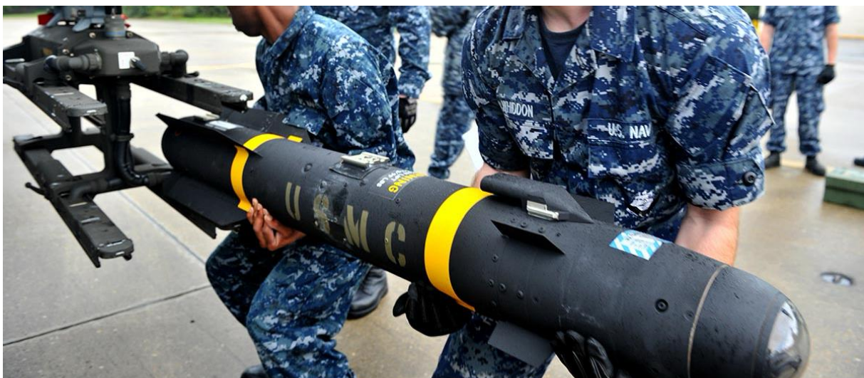
An Hellfire missile being fixed on a U.S. Navy helicopter wing. At the nose of the missile is the seeker system, or laser seeker. Behind it are the warhead, the fuze, guidance, gyro, propulsion and control. Military.com, https://www.military.com/equipment/agm-114-hellfire
