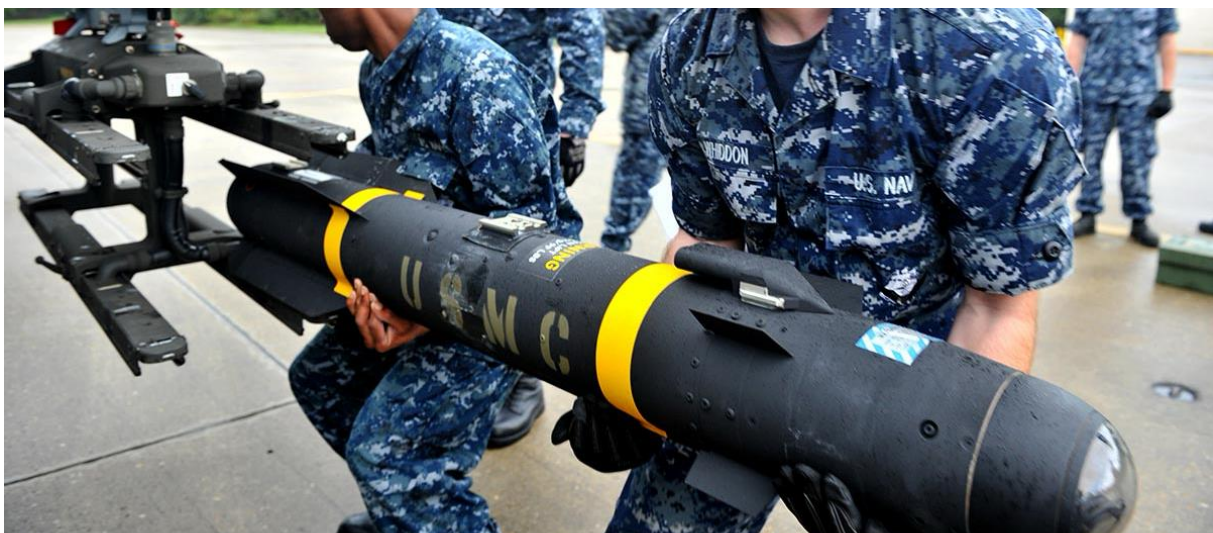
An Hellfire missile being fixed on a U.S. Navy helicopter wing. At the nose of the missile is the seeker system, or laser seeker. Behind it are the warhead, the fuze, guidance, gyro, propulsion and control. Military.com, https://www.military.com/equipment/agm-114-hellfire
