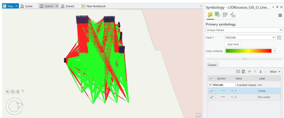
Figure E18 View of the conduction of LOS analysis in the 3D model of the Throne Room complex, with the 3d feature hidden. Green lines indicate visible distance to target points, while red the no visible. Symbology pane on the right indicates the values of the lines of sight. ArcGIS Pro, Local Scene. (Figure: V. Georgiopoulou).
