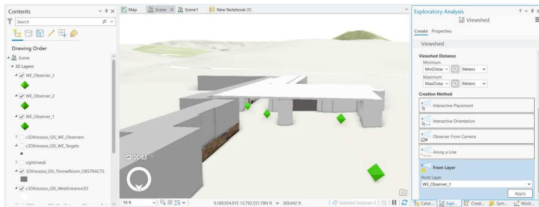
Figure 4.1.13 View of the observer points saved as a layer for the conduction of Exploratory Viewshed Analysis in the 3D model of the West Entrance complex. ArcGIS Pro, Local Scene. (Figure: V. Georgiopoulou).
