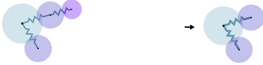
Figure 16: Illustration of protrusion retraction. The algorithm for protrusion retraction: (1) Choose a protrusion to be decreased in size. (2) The tip segment of this protrusion decreases in size. (3) If this decrease makes the tip segment radius less than a certain minimum radius threshold, the number of particles decreases as the tip particle and all of its bonds are removed. Then, the volume of the tip particle is reincorporated into the main cell, which grows to compensate.
