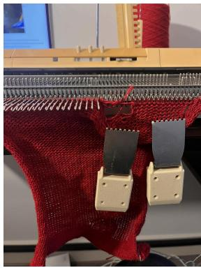
Figure 2: Knitting a sock on my knitting machine. Some stitches from the heel have inexplicably fallen off the needles. Photo taken by author.
