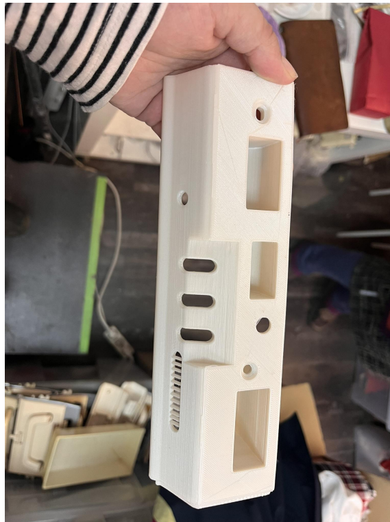
Figure 6: A 3D printed, modified cover for an electronic knitting machine. The cover allows for space for more tools and the AYAB hack. Printed by Victoria, photo taken by author at ETIB.
