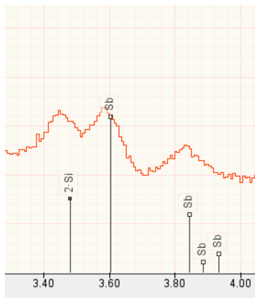
Figure 4.6: Identified Si K \alpha K sum peak adjacent to the Sb L \alpha peak.
