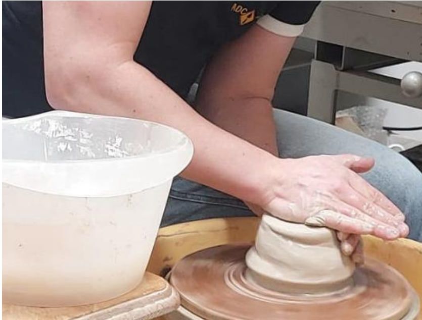
Figure 16: P2 performs a coning movement, pictured pressing downward a cone, to further homogenize the clay. Note that P2 is leaning one elbow against the leg for extra support.
