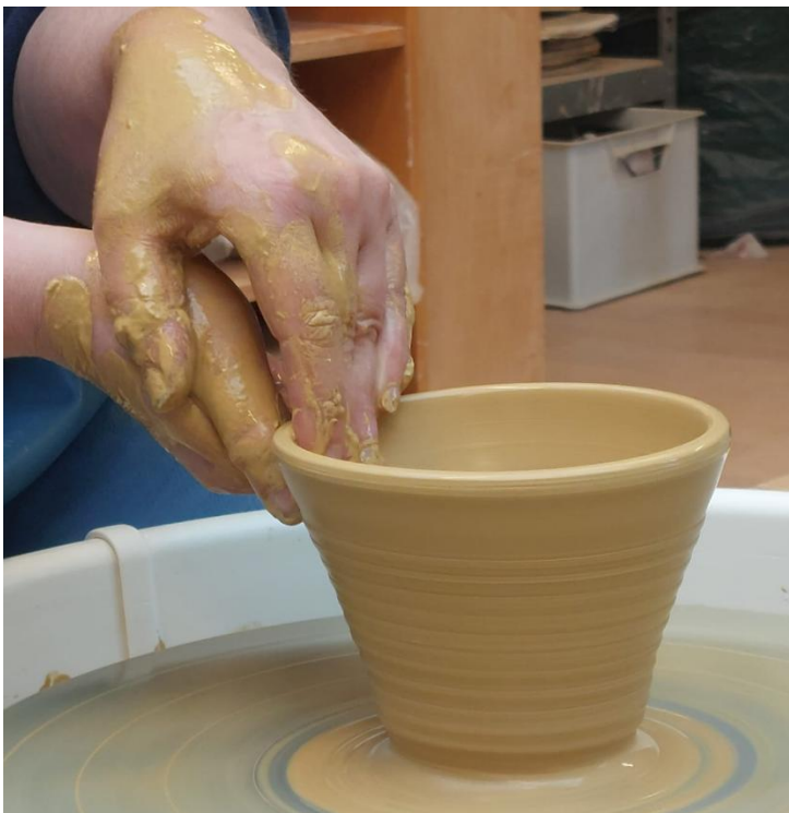
Figure 30: P5 lifts up the wall in a calm, controlled manner, creating a wall as even as possible, ensuring the hands are touching at all times to estimate the distance between the fingertips.
