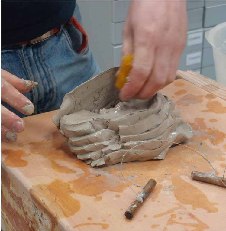
Figure 14: P2 adds water to the clay while in the process of wedging. The clay hump is alternatively wedged, cut into slices using a wire cutter to add water, and wedged again, until the desired plasticity has been reached.
