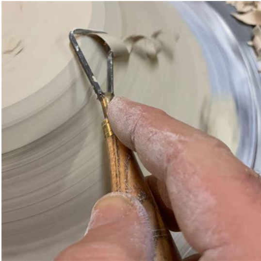
Figure 44: A demonstration of the use of an iron potter's trimming tool. Note that the open shape allows the trimmed clay to be guided off the clay so as to not interfere with further trimming. (Picture taken by potter Gary Jackson and published on www.firewhenreadypottery.com ).
