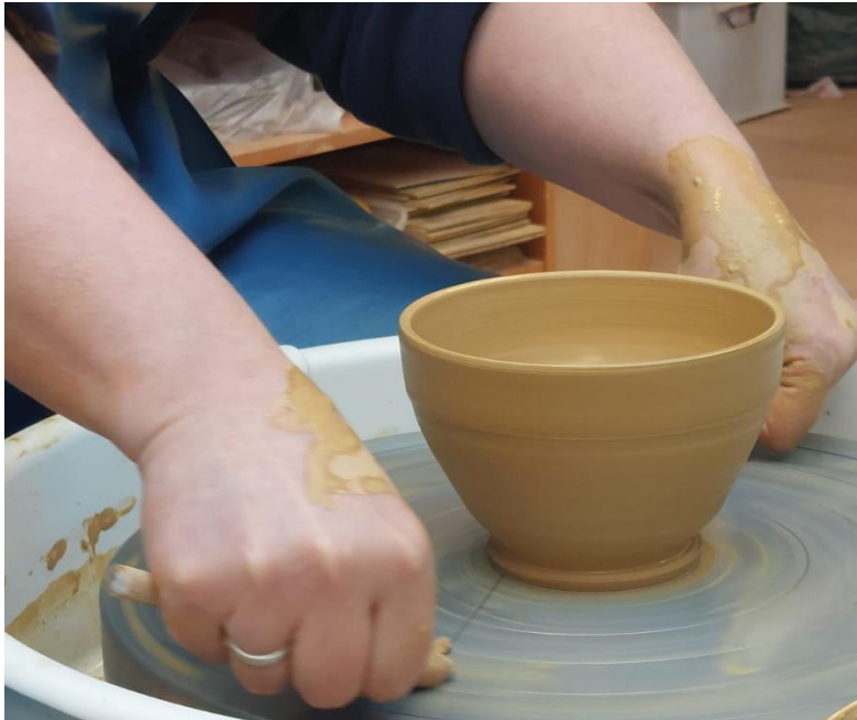
Figure 39: P5 uses a wire cutter to slice the vessel from the wheel, slicing away from the body.
