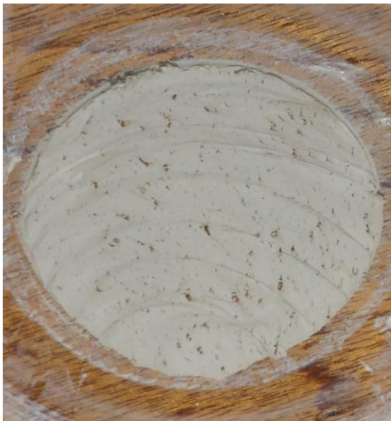
Figure 40: P2 has sliced the vessel off the wheel using a wire cutter slicing towards the body, leaving behind dragging traces in the clay left on the wheel. P2 explained that at different points in time, potters would prefer to either slice in one motion, or in a zigzagging motion like P2 did here.
