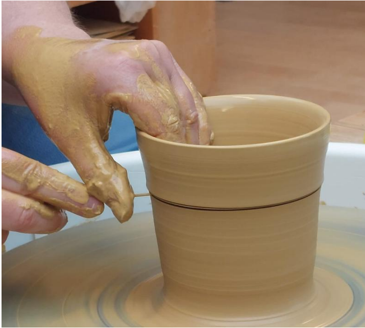
Figure 34: P5 trims the top part of the wall of the wall to create a horizontally even rim and get rid of excess clay using a potter's needle. This picture was taken in early wet forming while still forming the wall, as opposed to Figure 33 that was taken towards the end of primary forming.
