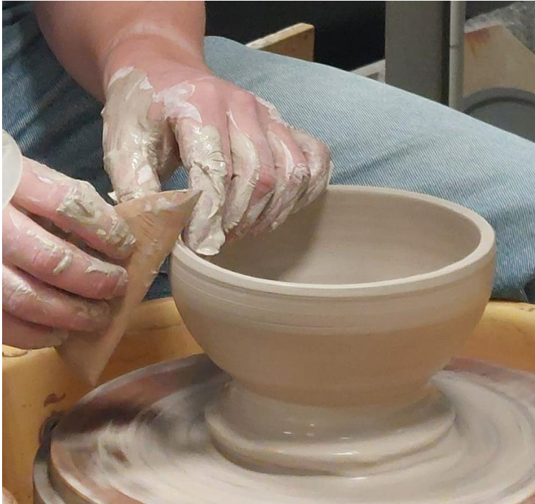
Figure 35: P2 uses a wooden scraper to shape and smoothen the wall towards the end of the secondary wet forming stage, moving upwards the slip layer that has collected at the lower outside part and the wall.
