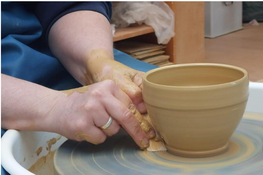
Figure 38: P5 uses a plastic scraper to clean the wheel and the bottom part of the vessel from excess slip.
