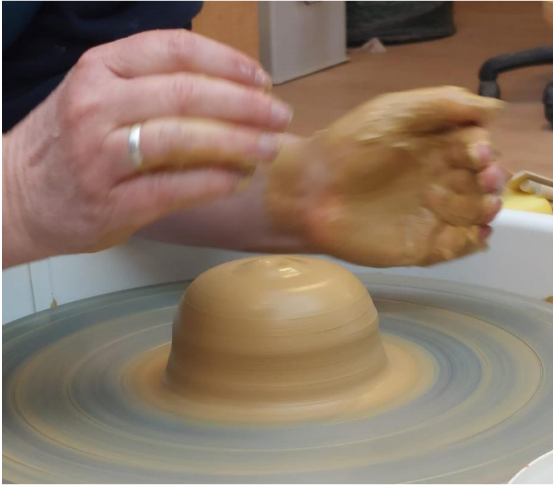
Figure 18: Just like P2, P5 creates a prebuilding shape resembling a flattened pot upside down in preparation for the basic bowl shape of the Frisian candle holder.
