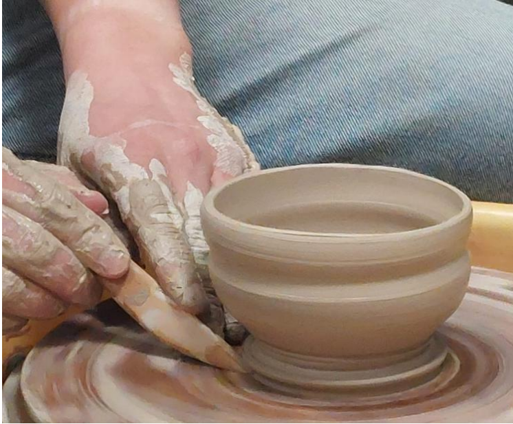
Figure 37: P2 cleans the lower part of the vessel using a wooden potter's spatula. This picture was not taken during the production process of the Frisian candle holder replica, but during a production process started by P2 using left-over clay directly after finishing the candle holder.
