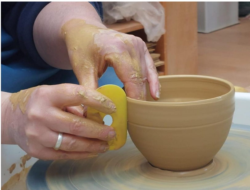
Figure 36: P5 uses a plastic scraper to shape and smoothen out the wall towards the end of the secondary wet forming stage, moving upwards the slip layer that has collected at the lower outside part and the wall and ensuring the hands are touching each other at all times.
