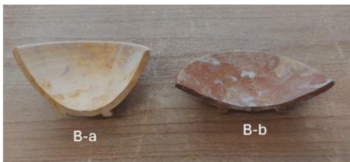
Figure 20: Demonstration material in P5's workshop to help explain different forming trajectories of different vessel shapes. B stands for bowl, of which B-a and B-b demonstrate different versions. Both feature a connected tension arch, creating a downward parabola shape. B-b showcases how choices in forming trajectories of a bowl and a plate can be placed on a spectrum.
