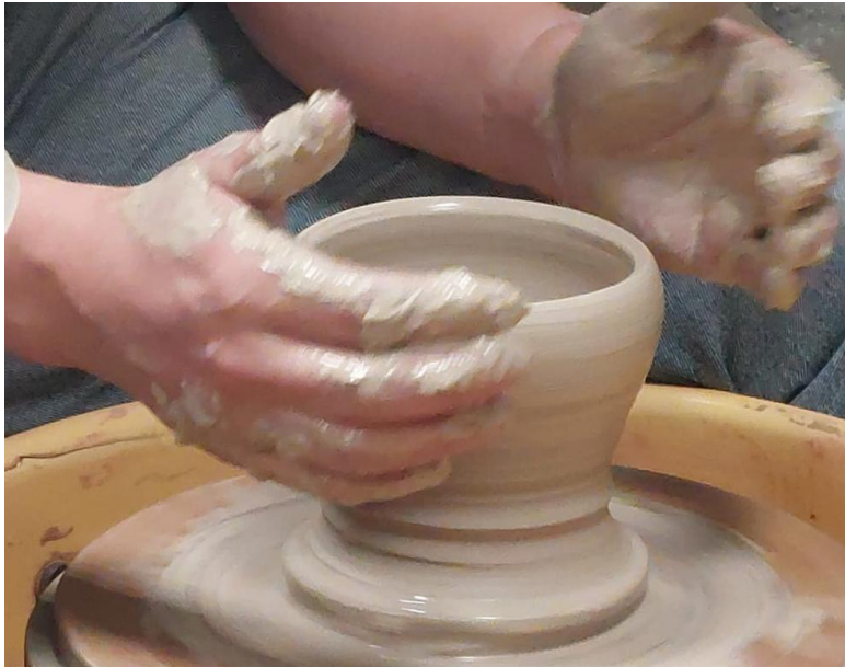
Figure 31: P2 is in the process of lifting up unnecessary supporting clay into the wall, while shaping the wall more into the final shape of the Frisian candle holder.
