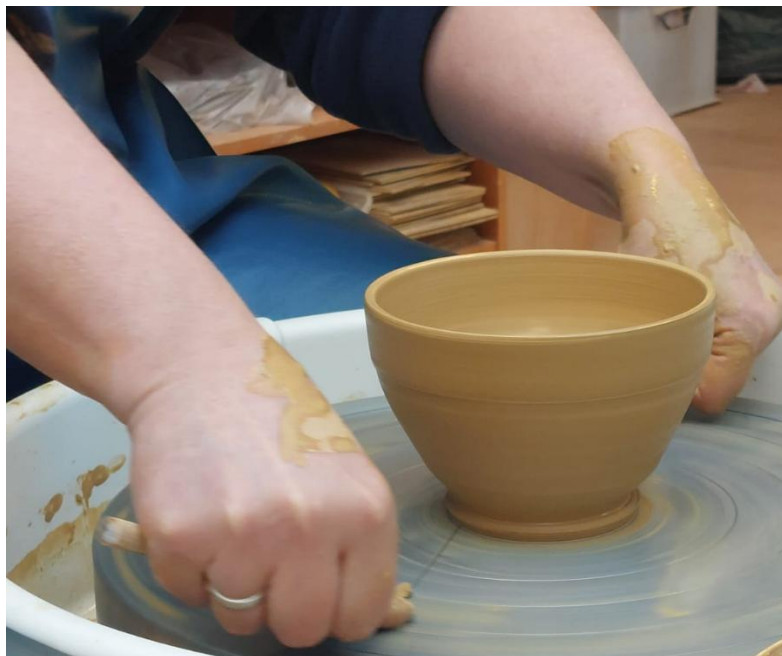
Figure 39: P5 uses a wire cutter to slice the vessel from the wheel, slicing away from the body.
