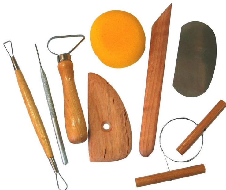
Figure 13: An example of a basic potter's toolkit. From left to right: an iron trimming tool, an iron potter's needle, a larger iron trimming tool, a wooden scraper, a soft-edged sponge, a wooden potter's spatula, a wire cutter, and a metal scraper. Trimming tools, spatulas and scrapers exist in many different shapes and sizes; the choice of which one to use when often depends on personal preference of the potter. (Public product marketing picture found on www.cavalierart.com ).
