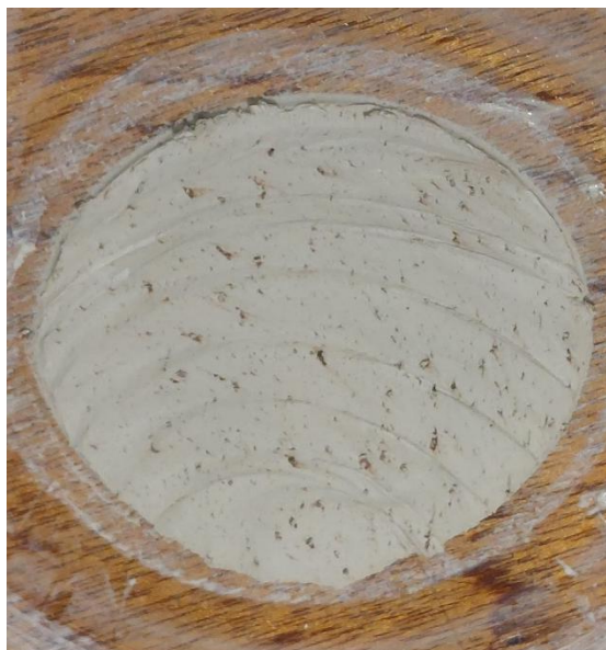
Figure 40: P2 has sliced the vessel off the wheel using a wire cutter slicing towards the body, leaving behind dragging traces in the clay left on the wheel. P2 explained that at different points in time, potters would prefer to either slice in one motion, or in a zigzagging motion like P2 did here.
