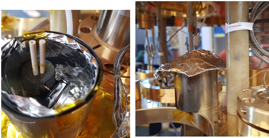
Figure 3.4: The trap in its shielding (L) and the shielding with lid (R)
