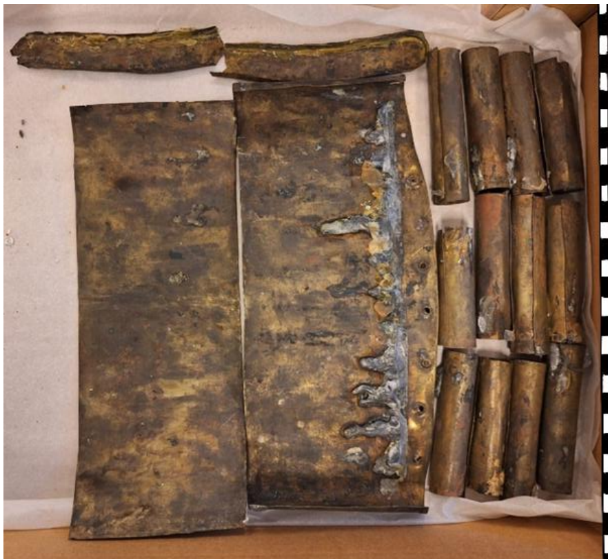
Fig. 3.1.1 A broken cartridge case. The state of the case handily shows all the individual components. Photograph: A. Treurniet. (Scheepvaart Museum Amsterdam, Object ID A.4714(07)09, https://collectie.hetscheepvaartmuseum.nl/details/museum/508048 ).
