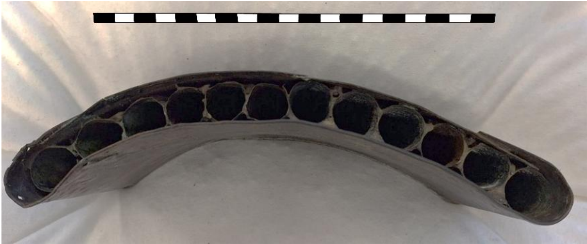
Fig. 3.1.3 The copper components of a cartridge case put together, as seen from the top. The image has been brightened for better visibility. Photograph: A. Treurniet. (Scheepvaart Museum Amsterdam, Object ID A.4714(07)03, https://collectie.hetscheepvaartmuseum.nl/details/museum/508042 ).
